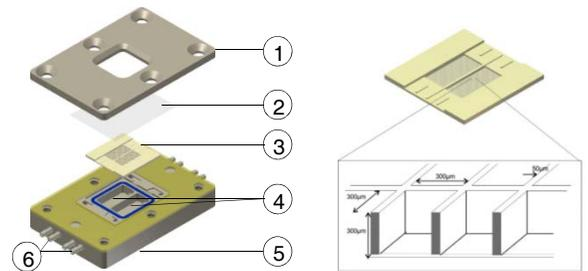
Figure 1: Left: Exploded view of a 3<sup>D</sup>-KITChip-containing MRI-compatible bioreactor. 1=upper lid, 2=microscope cover slip, 3=3<sup>D</sup>-KITChip, 4=independently perfused compartments, 5=bioreactor housing, 6=connection for perfusion. Right: 3<sup>D</sup>-KitChip with flat bottom (f-3<sup>D</sup>-KitChip) in detail.
