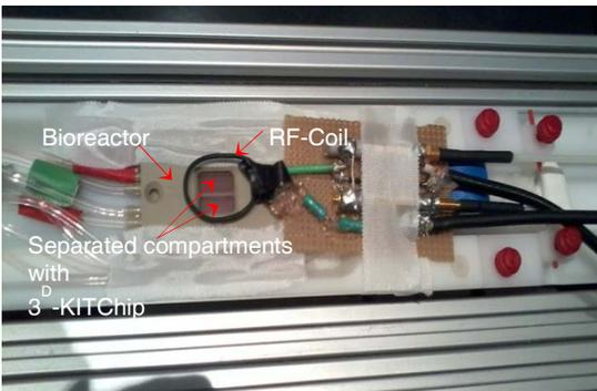
Figure 2: Bioreactor with custom made <sup>23</sup>Na surface
