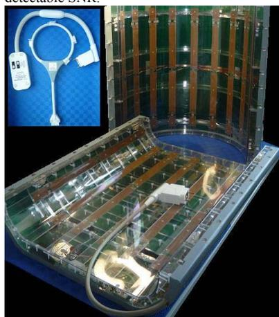
Figure 1: <sup>23</sup>Na asymmetric birdcage resonator and receive-only surface coil with preamplifier-holding adapter box (inset).
